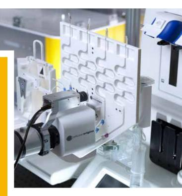
Through precise robotic handling, and full digital control and traceability, Constellation automates complex processes and distinct unit operations, and the connection between them, with full reproducibility. It does this physically with accurate handling, precise fluid transfer and automated sterile connections.
